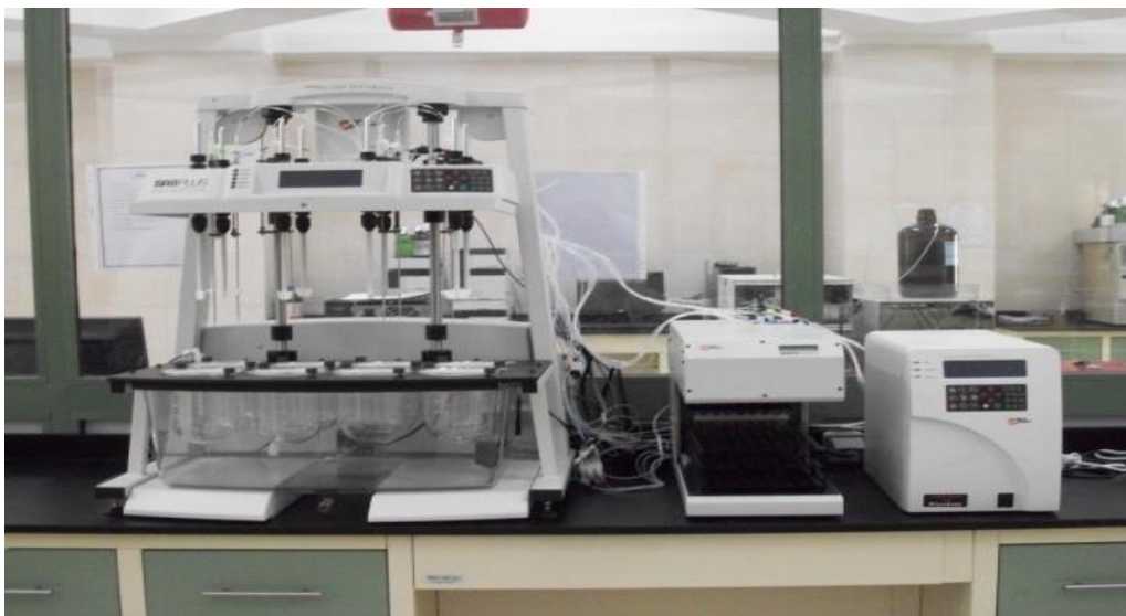
Fully programmed dissolution apparatus Contains eight 1 liter cups and equipped with auto sampler to save time and improve performance
